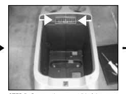
**STEP 5:** Remove the armrest lid of the console by removing four Phillips head screws.
